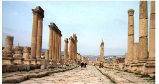
about paving stones laid diagonally so as not to trap chariots' wheels and the origin of our standard road width (18') to let two chariots pass. The underground storm drainage system reminded me of how long it took us to re-invent what the Roman engineers already knew!
